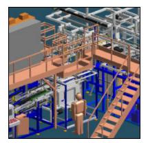
designed this machine in the same amount of time with 2D CAD, but because of all the moving parts there would have been many errors," says vice president Steve Cook. "Fixing those errors would have taken us at least another year. By building the machine digitally using the software's assembly modeling capability, we knew everything would fit. That was much more efficient than tearing apart a prototype to make it work."
